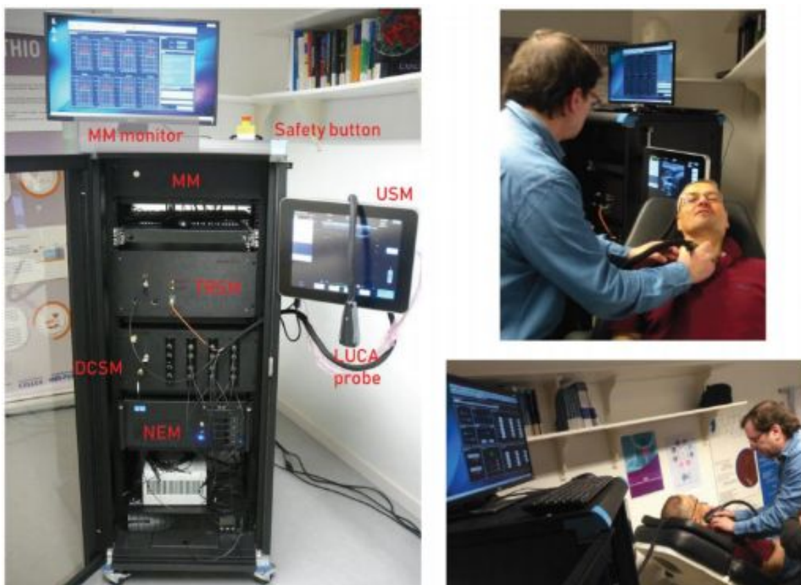
Figure 1: The fully functional LUCA demonstrator prototype (left, as reported in D3.5) at an initial practical testing session (right).
